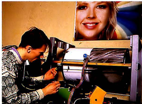
■ Sandy tinkers with the drum of the printer. Note the bicycle chain which pulls the airbrush along.
